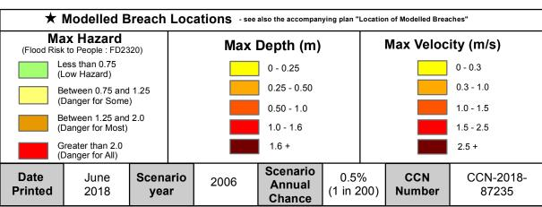
The map is based on computer modelling of simulated breaches at specific locations. Each breach has been modelled individually and the results combined to create this map. Multiple breaches, other combinations of breaches, different sized tidal surges or flood flows may all give different results.
