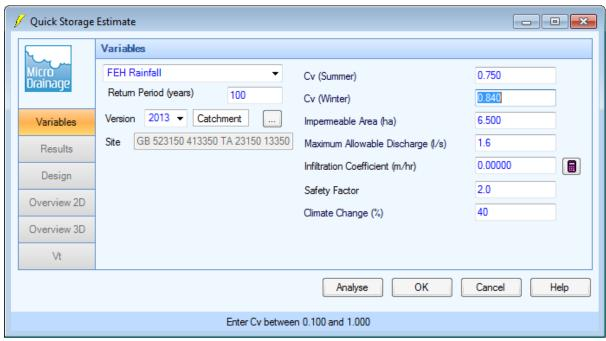
Figure 4: Source Control Input for Greenfield Run-off Discharge Rate
